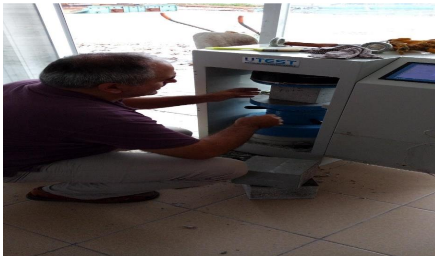
Figure 1. Cube compressive strength test
