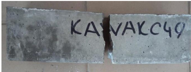
Figure 7. Prismatic specimen broken after test
