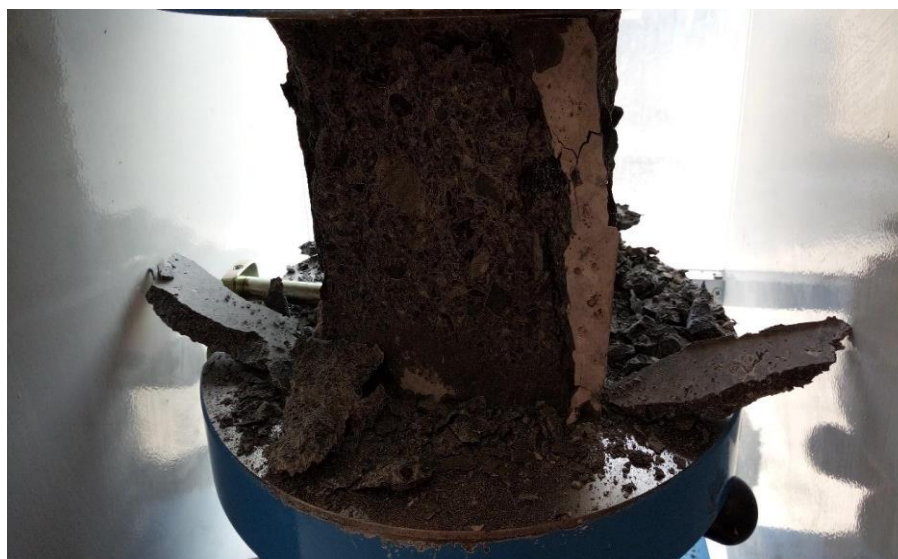
Figure 2. Cube sample fracture
